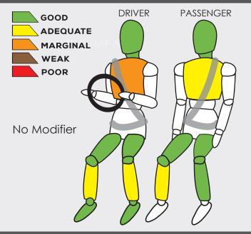
The SUV's frontal occupant compartment remained stable in the frontal offset test. Data obtained from the test dummy showed there was marginal protection to the driver's chest. In addition, both of the driver's lower legs and the passenger's right lower leg received adequate protection in the test.
