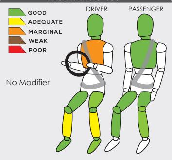
SUV's frontal occupant compartment remained stable in the frontal offset test. Data obtained from the test dummy showed there was marginal protection to the driver's chest. In addition, both of the driver's lower legs received adequate protection in the test. SIDE IMPACT
