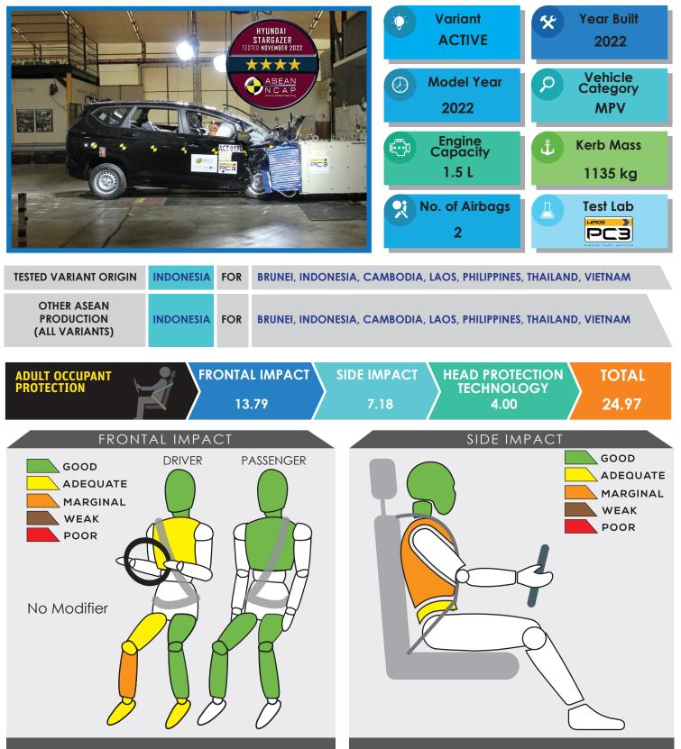
Data obtained from the tested dummy showed there is high possibility for the driver to sustain injuries to the chest and its right leg in a real world crash. Nevertheless, the MPV's frontal occupant remained stable in the frontal offset test. The driver received marginal protection to the chest during the side impact test.
