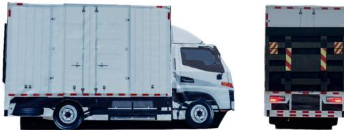
Figure 9 Soft light-truck target
