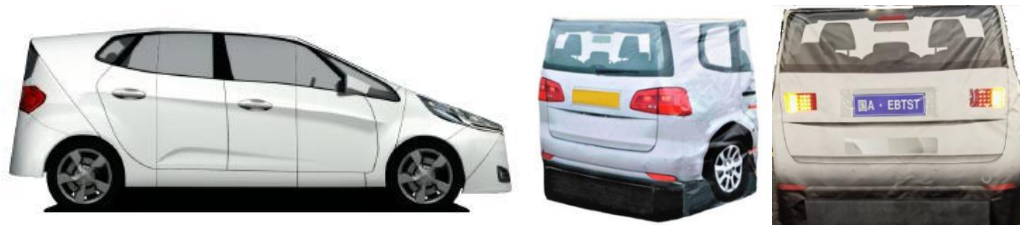
Figure 4 Soft passenger car target (3D full-vehicle target without a lighting system and with a lighting system)
