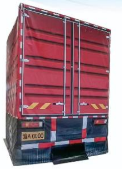
Figure 8 Soft heavy-truck target
