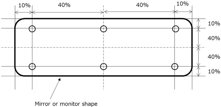
Figure 4: Measurement points location of mirror or monitor surface
