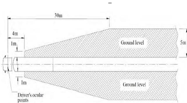
New regulation for reversing motion (Rear indirect vision, rear view camera)
