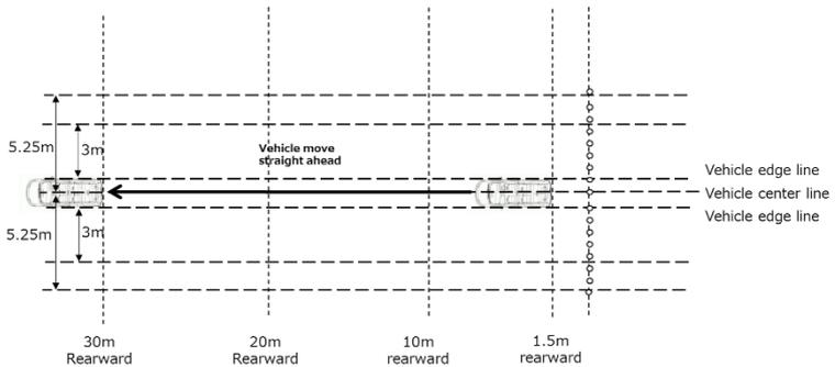
Figure 3: Actual movement of vehicle in the test
