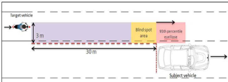
Figure 3-2: Must not give blind spot warning to the driver
