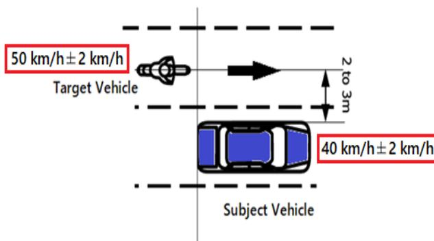
Figure 3-1: Target Vehicle overtaking Subject Vehicle speed
