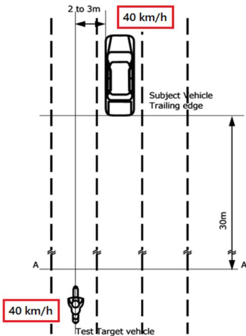
Figure 2-1: Target Vehicle entering 30-meter zone with steady speed
