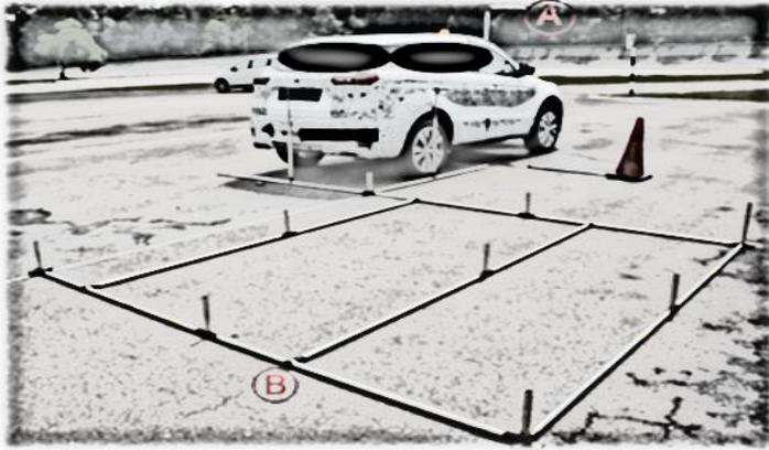
Figure 1-1: Blind spot zone setup
