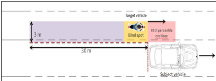
Figure 3-4: Must give blind spot warning to the driver
