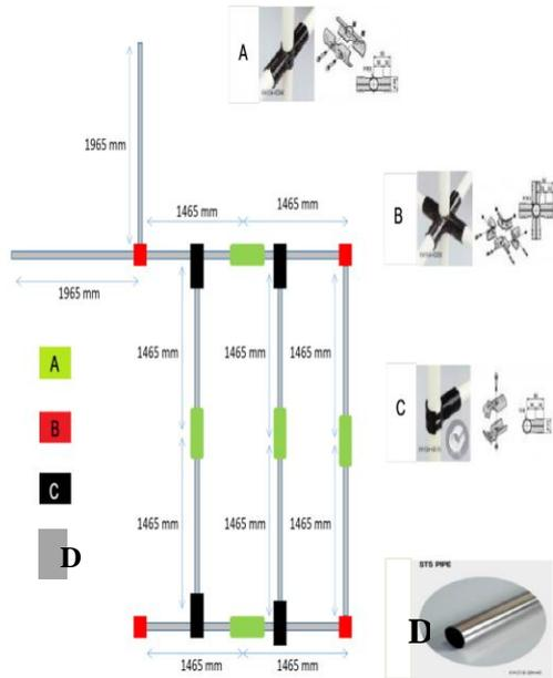
Figure 1-2: Blind spot coverage zone jig
