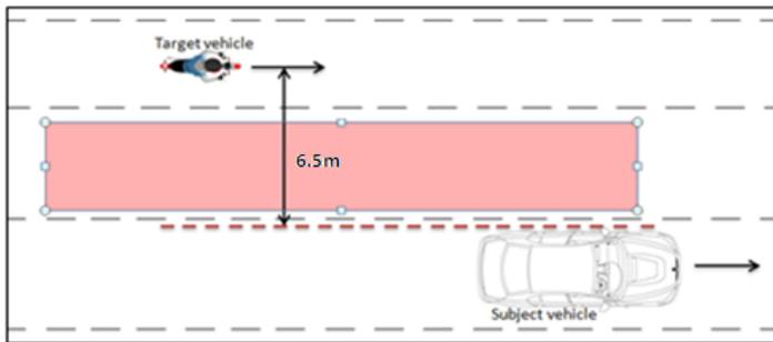
Figure 3-5: Target vehicle shall be maintained at 6.5 meters during test
