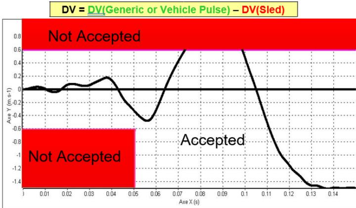
Sample pulse showing a sled test that cannot be accepted as parts of DV are outside the acceptable zone
