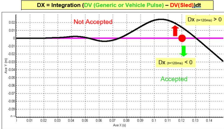
Sample picture shows a sled test that cannot be accepted as DX is positive @ 120 ms
